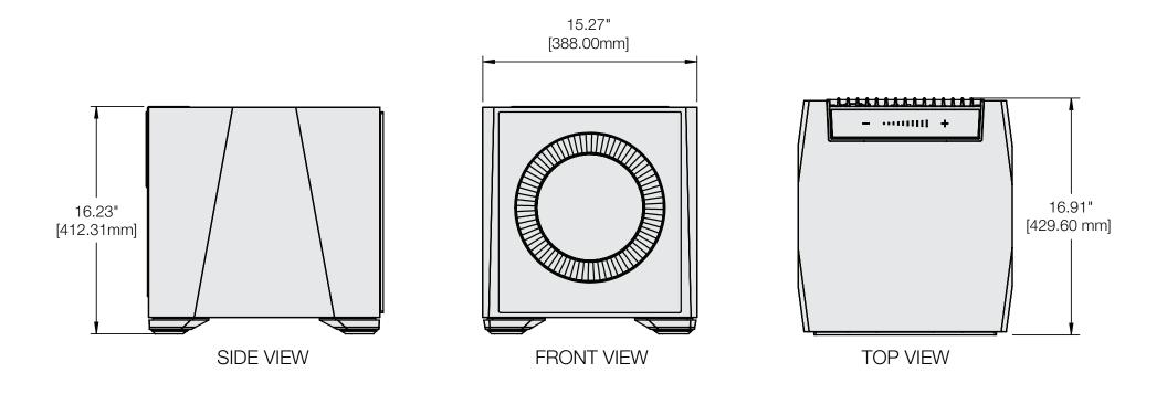
OVERALL DIMENSIONS\*: (H) 16.23" [412.31mm] x (W) 15.27" [388mm] x (D) 16.91" [429.60mm] WEIGHT: 65.1lbs (29kg) each
